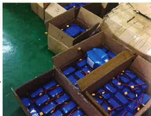
Poor quality lithium battery packed with unsafe packaging
